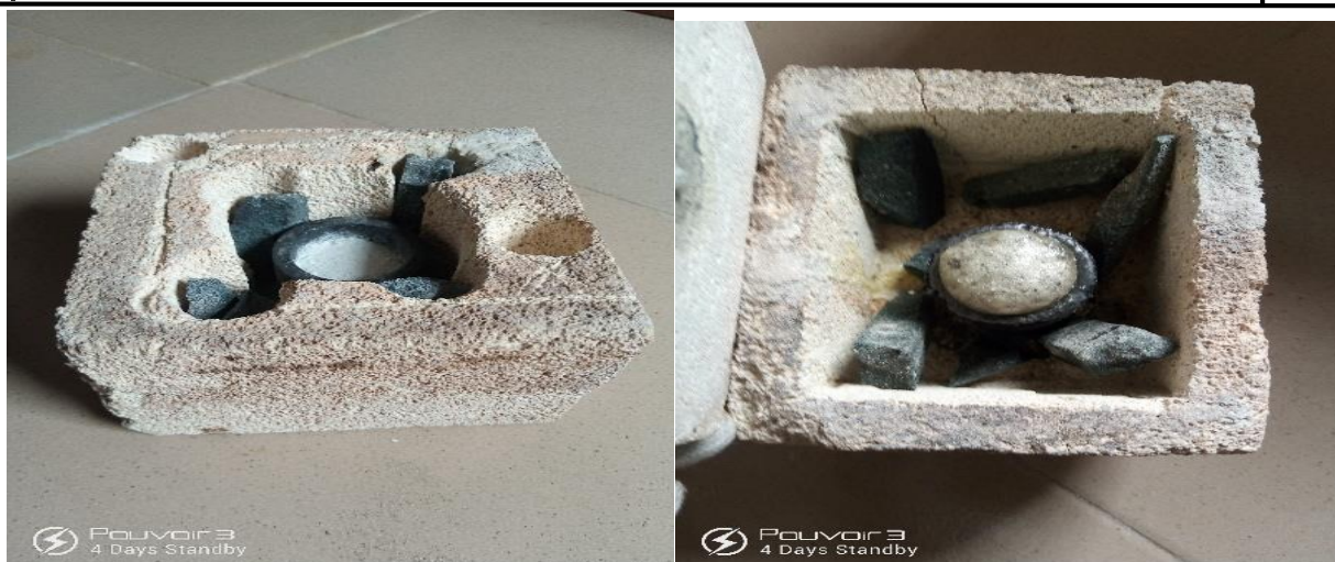
Figure 2: a fabricated kiln pot laced with silicon carbide and graphite pot crucible filled with the batch to be charged into the microwave oven.
