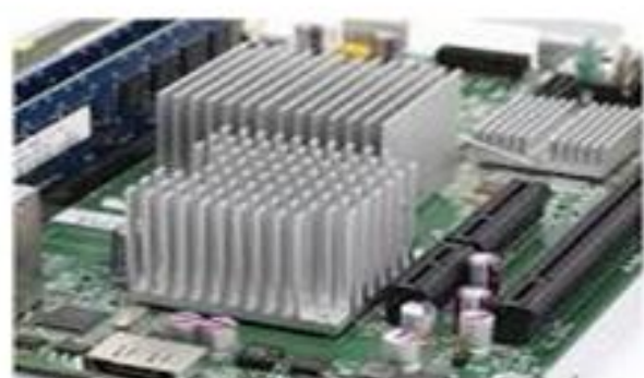
Plate 1: Heat sink for heat absorption
