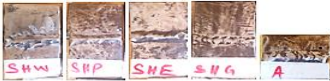
Figure 1: The experimental procedure shows an array of specimens after the SMAW welding operation.
