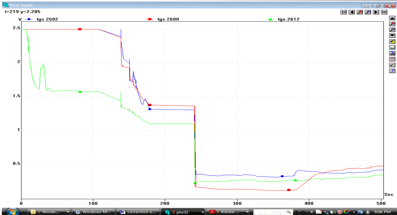
Figure 15: test with Ethanol when the load resistor is 25kΩ
